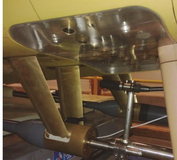
**Figure 1:** Aft shaft bracket and the wakefield measurement equipment fitted with a hydrophone and the perspex block with the pressure transducers forming the array.
